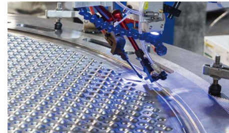
Plate welding equipment
