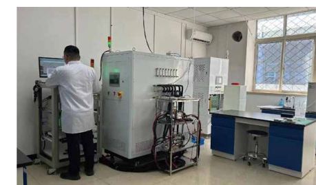
PEM Electrolytic Water Testing Platform
