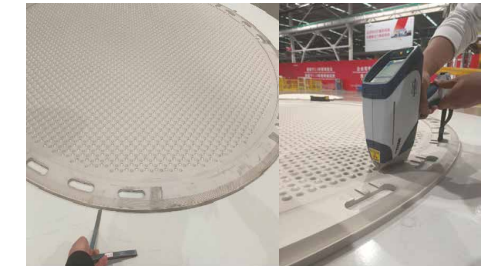
Flatness and Coating Testing
